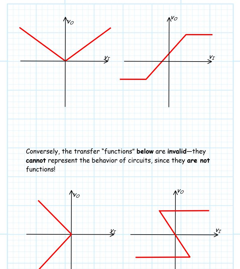
Moreover, we find that **circuit** transfer functions must be **continuous**. That is,  $v_O$  **cannot** "instantaneously change" from one value to another as we increase (or decrease) the value  $v_I$ .
