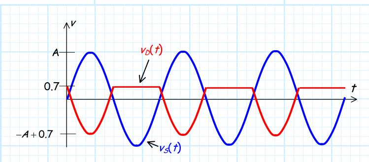
Note that this minimum diode voltage is very negative, with an absolute value ( $|v_D^{min}| = A - 0.7$ ), approximately equal to the value of the source magnitude A.
