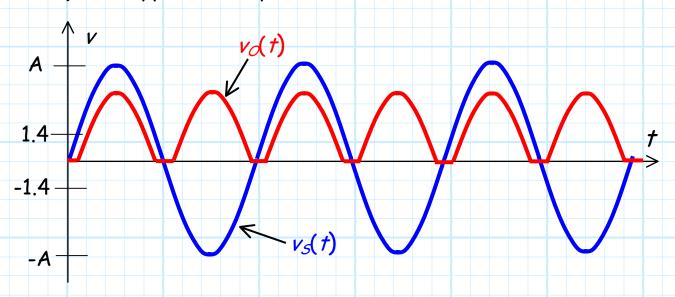
We see that the junction diode bridge rectifier output is very close to ideal. In fact, if A>>1.4 V, the DC component of this junction diode bridge rectifier is approximately:
