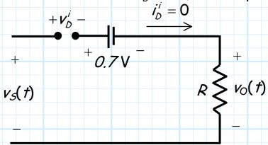
Q: Fascinating! The output voltage is zero when the ideal diode is reverse biased. But, precisely when is the ideal diode reverse biased? For what values of  $v_s$  does this occur?
