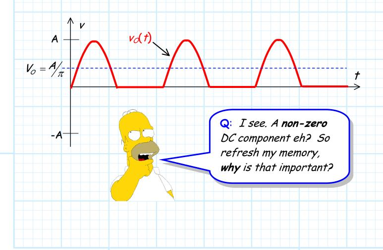
A: Recall that the power distribution system we use is an AC system. The source voltage  $v_s(t)$  that we get when we plug our "power cord" into the wall socket is a 60 Hz sinewave—a source with a zero DC component!
