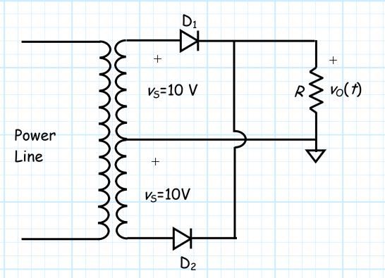
Conversely, if  $v_S$ =-10 V, the anode of  $D_1$  will be 10V **below** ground potential (i.e., -10V), while the anode of  $D_2$  will be 10V **above** ground potential:
