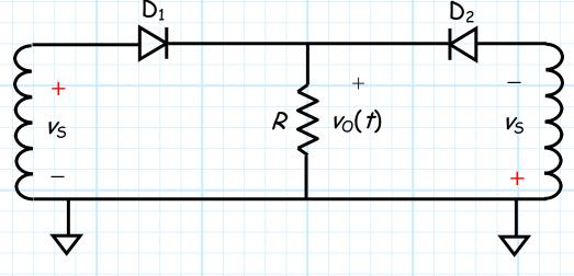
Note that the secondary voltages at either end of this circuit are the **same**, but have **opposite** polarity. As a result, if  $v_5$ =10, then the anode of diode  $D_1$  will be 10 V **above** ground, and the anode at diode  $D_2$  will be 10V **below** ground—just like before!
