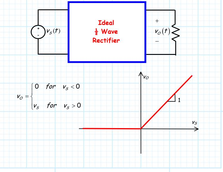
Pretty simple! When the input is negative, the output is zero, whereas when the input is positive, the output is the same as the input.
