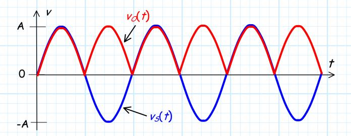
Again we see that the junction diode full-wave rectifier output is **very close** to ideal. In fact, if A>>0.7 V, the **DC** component of this junction diode full wave rectifier is approximately:
