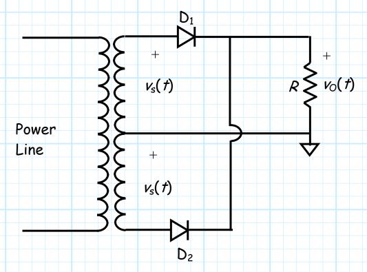
Note that we are using a **transformer** in this circuit. The job of this transformer is to **step-down** the large voltage on our power line (120 V rms) to some **smaller** magnitude (typically 20-70 V rms).
