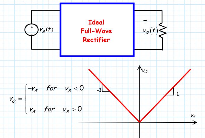
If the ideal half-wave rectifier makes negative inputs zero, the ideal full-wave rectifier makes negative inputs—positive! For example, if we again consider our sinusoidal input, we find that the output will be:
