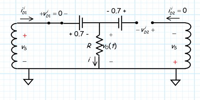
Note that we need to determine 3 things: the ideal diode current  $i'_{D1}$ , the ideal diode voltage  $v'_{D2}$ , and the output voltage  $v_{O}$ . However, instead of finding numerical values for these 3 quantities, we must express them in terms of source voltage  $v_{S}$ !
