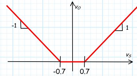
The output of this full-wave rectifier with a sine wave input is therefore:
