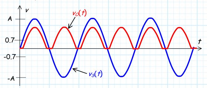
Note how this compares to the transfer function of the ideal full-wave rectifier:
