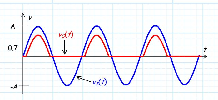
Although the output is **shifted downward** by 0.7 V (note in the plot above this is **exaggerated**, typically A >> 0.7V), it should be apparent that the **output** signal  $v_{c}(t)$ , unlike the input signal  $v_{c}(t)$ , has a **non-zero** (positive) **DC** component.
