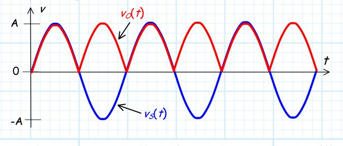
The result is that the output signal will have a DC component twice that of the ideal half-wave rectifier!
