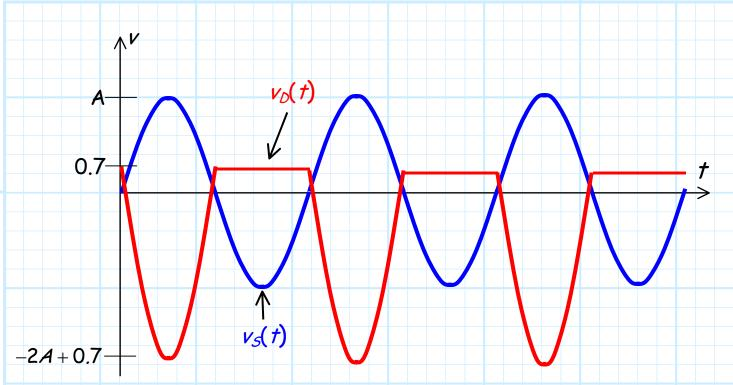
Note that this **minimum** diode voltage  $v_D$  is **very negative**, with an absolute value ( $|v_D^{min}| = 2A - 0.7$ ) nearly **twice** as large as the source magnitude A.
